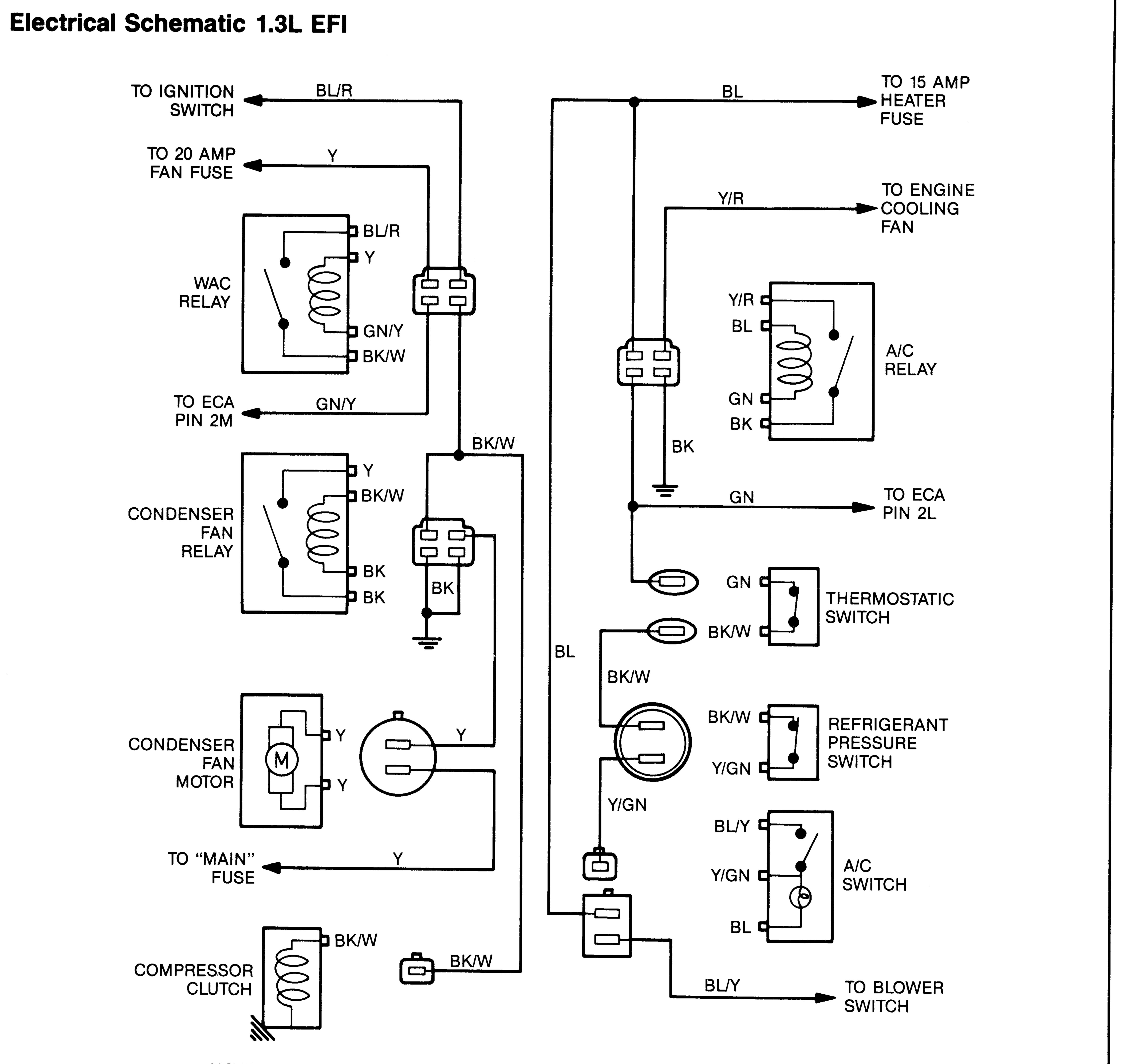
NOTE: WIRING SCHEMATIC SHOWS PIN OUT LOOKING INTO HARNESS CONNECTOR.
